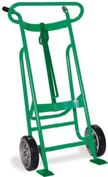
**2-Wheel EZY-Rol™ Automatic Drum Trucks** feature ValleyCraft's exclusive EZY-Tilt™ design and spring-loaded chime hook so the operator never has to touch the drum. Choice of steel or aluminum. Shoes adjust to handle 30- and 55-gal. drums up to 1,000 lbs. Available with optional hand brakes for added safety. Replaceable wheels, shoes and axles available. Five-chime hook and three-wheel options available.
